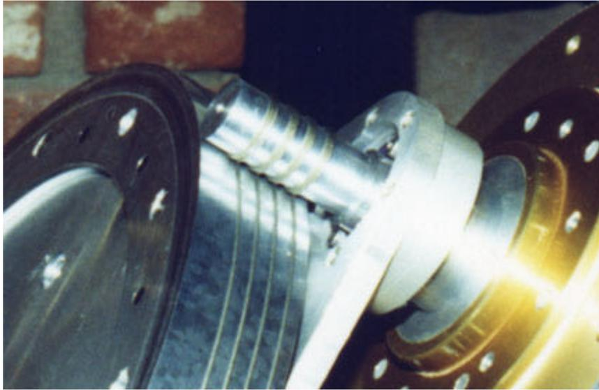
**View of cables wrapping around two shafts.**
